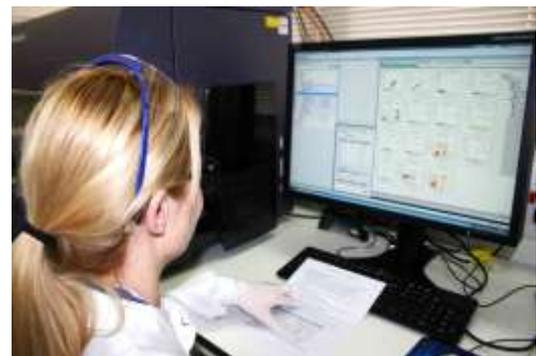
We use 2 Becton-Dickinson FACS CantoII, 8-colour, 3-laser, flow cytometer with 96 positions plate autoloader. Our IMag Cell Separation System augments the power of our flow cytometer, by enriching and depleting specific cell populations.
